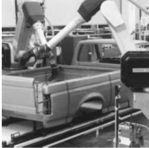
FIGURE 14.11.3 Robots inspect pick-up truck body prior to final assembly. (Courtesy of Fanuc Robotics, N.A.)
